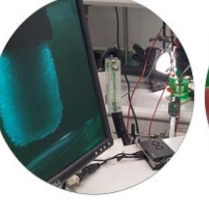
In situ monitoring of melt crystallization process using a modular camera system
