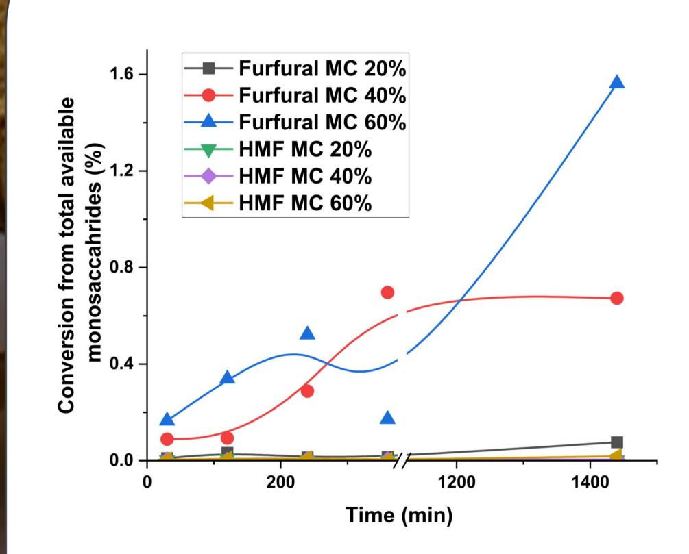
Degradation of monomeric sugars during gas hydrolysis. Degradation to HMF is negligible and conversion to furfural reaches 1.55% only at 60% moisture content and 24 h reaction time.
