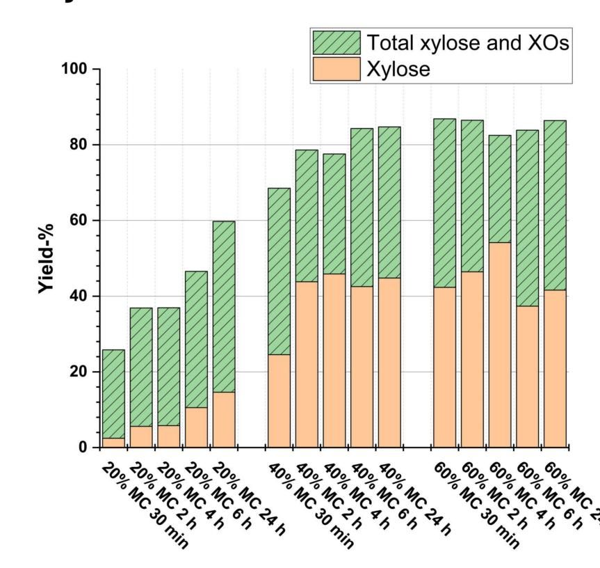
Yield of water-soluble xylose and xylose + xylooligosaccahrides (XO) from gas hydrolysis. In moisture contents of 40-60% around half of the hydrolyzed xylans are in monomeric form. Rest are different sized XOs. In 20 % moisture content most of the xylans are in oligosaccharide form.
