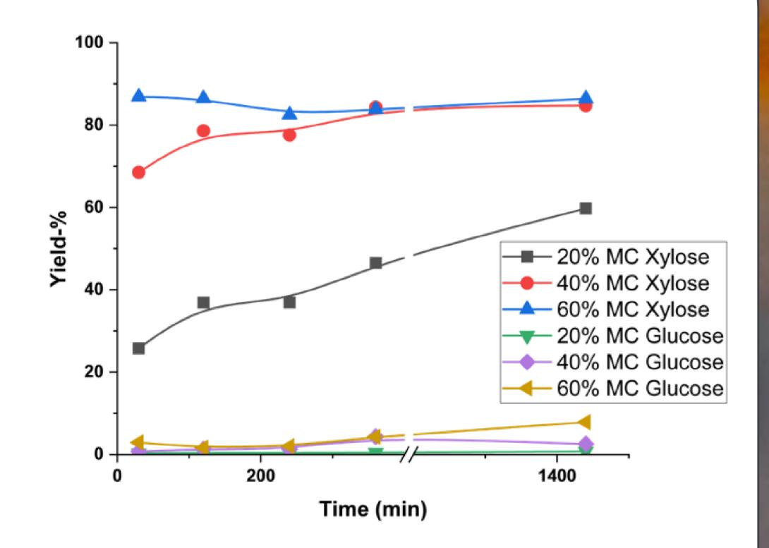
Total yields of water-soluble carbohydrates from prehydrolysis with hydrogen chloride gas. With all moisture contents mainly hemicellulose is degraded.
