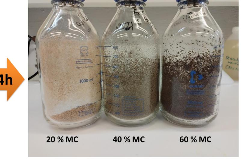
Samples after gas application and after 4 h reaction time prior to heating in water bath. None of the samples have turned into sticky syrup after 4 h reaction time.
