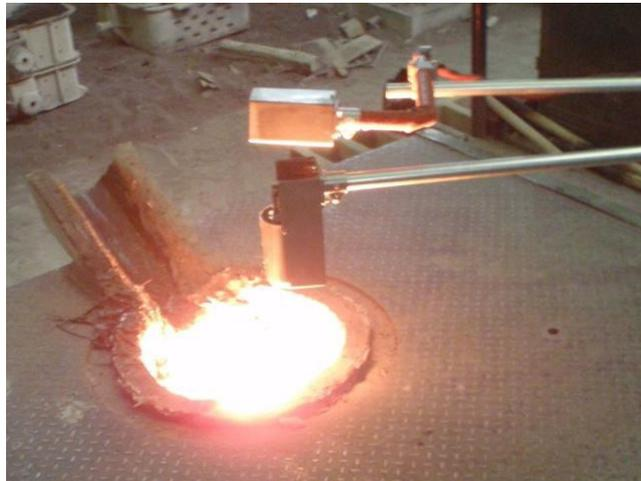
Figure 2: Trials at a foundry induction furnace containing liquid steel with the CE sensor (lower device) together with a housed camera for comparison (upper device)
