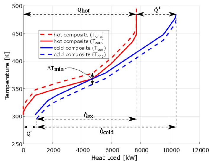
Figure 1: Hot and cold composite curves
