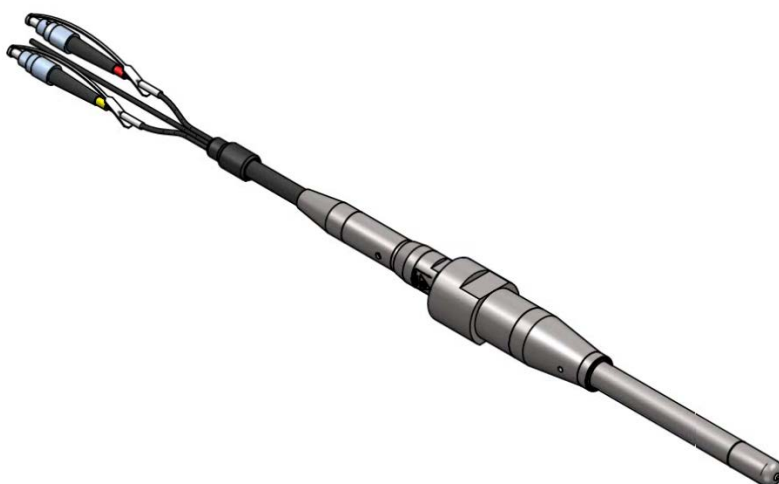
Figure 3: An image of Raman fibre optic probe used for in situ monitoring of emulsion polymerization within RECOBA demonstration.
