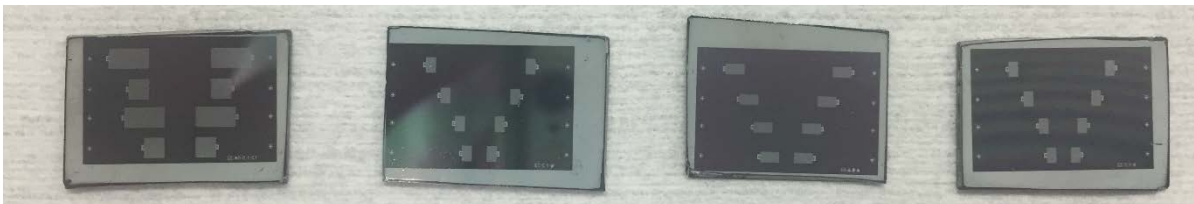
Figure 3 – Chips with SAW delay sensors using different geometries. Each chip contains four different sensors.
