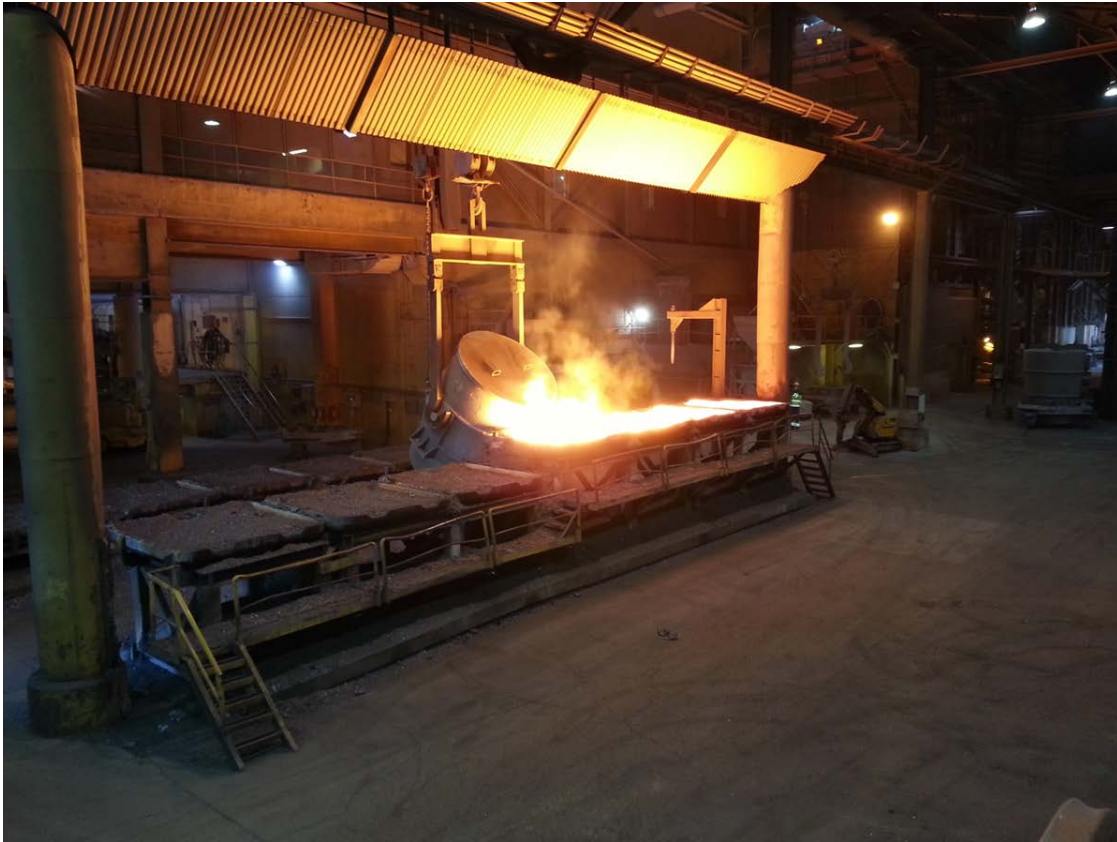
Figure 2 - Casting from a crane at Elkem Thamshavn.
