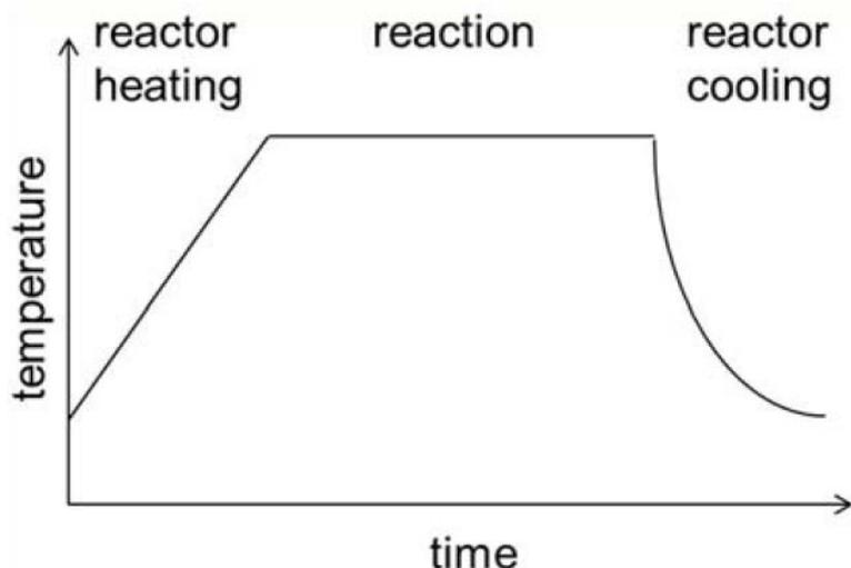
Figure 1: Example of batch reaction temperature
