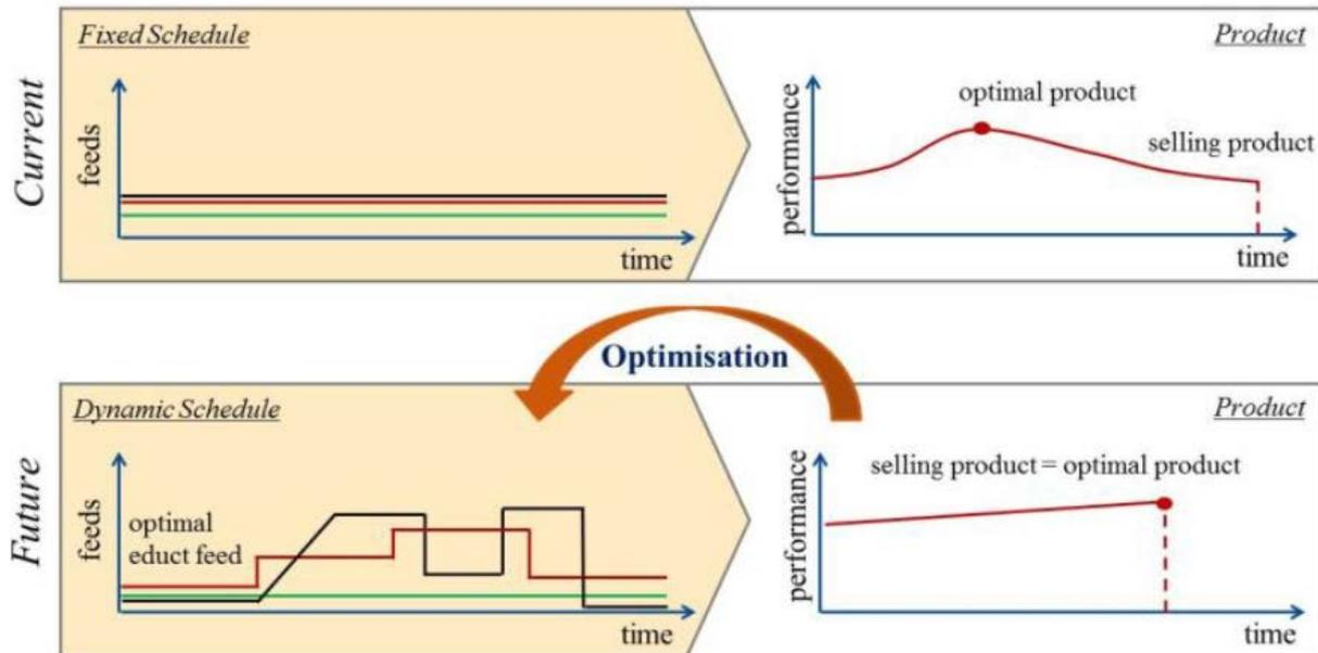
Figure 2: Advancing from time based recipes to state based process operation
