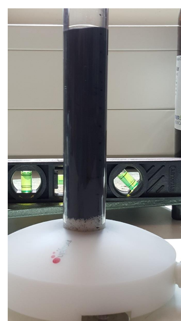
Fig. 1: Experimental set-up of the Expanded Bed Adsorption column
