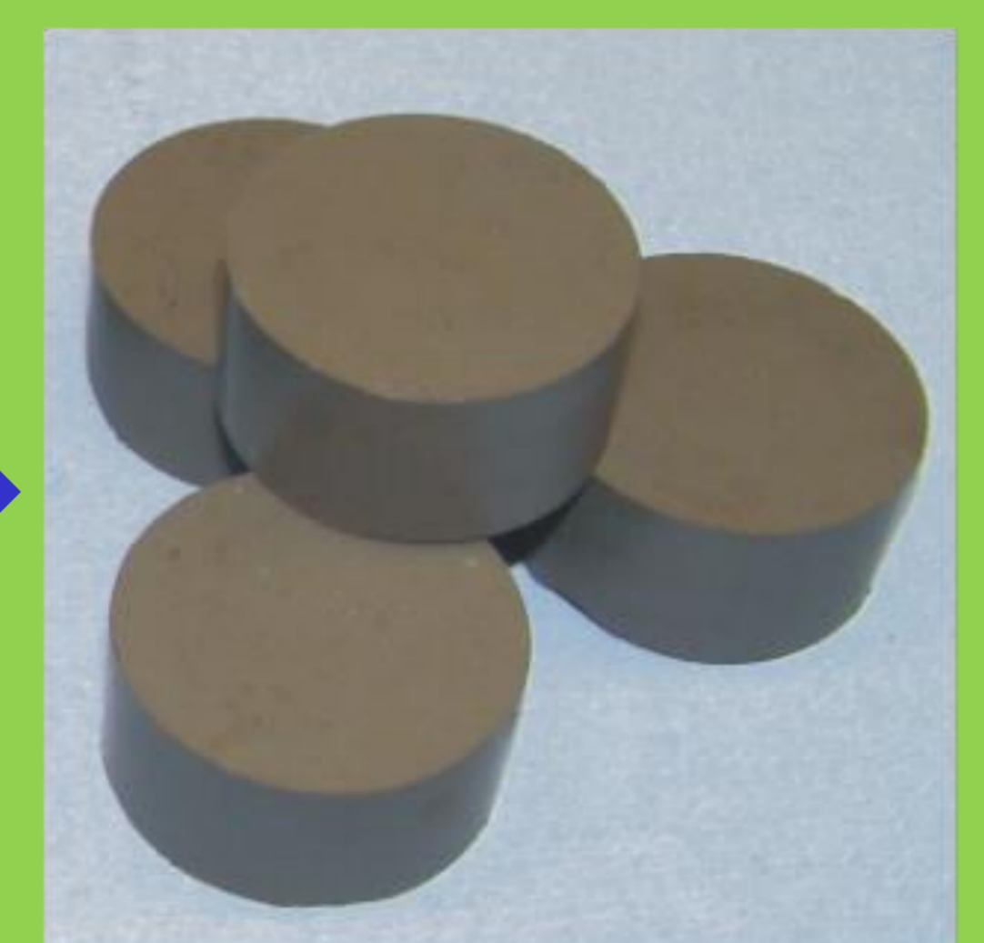
Removed scale after briquetting
