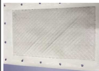
Fig. 2: No visible fouling effects after 2 weeks of operation
