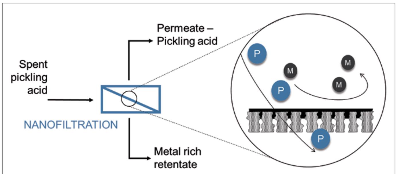
Figure 1: Scheme of P-recovery process at Sandvik
