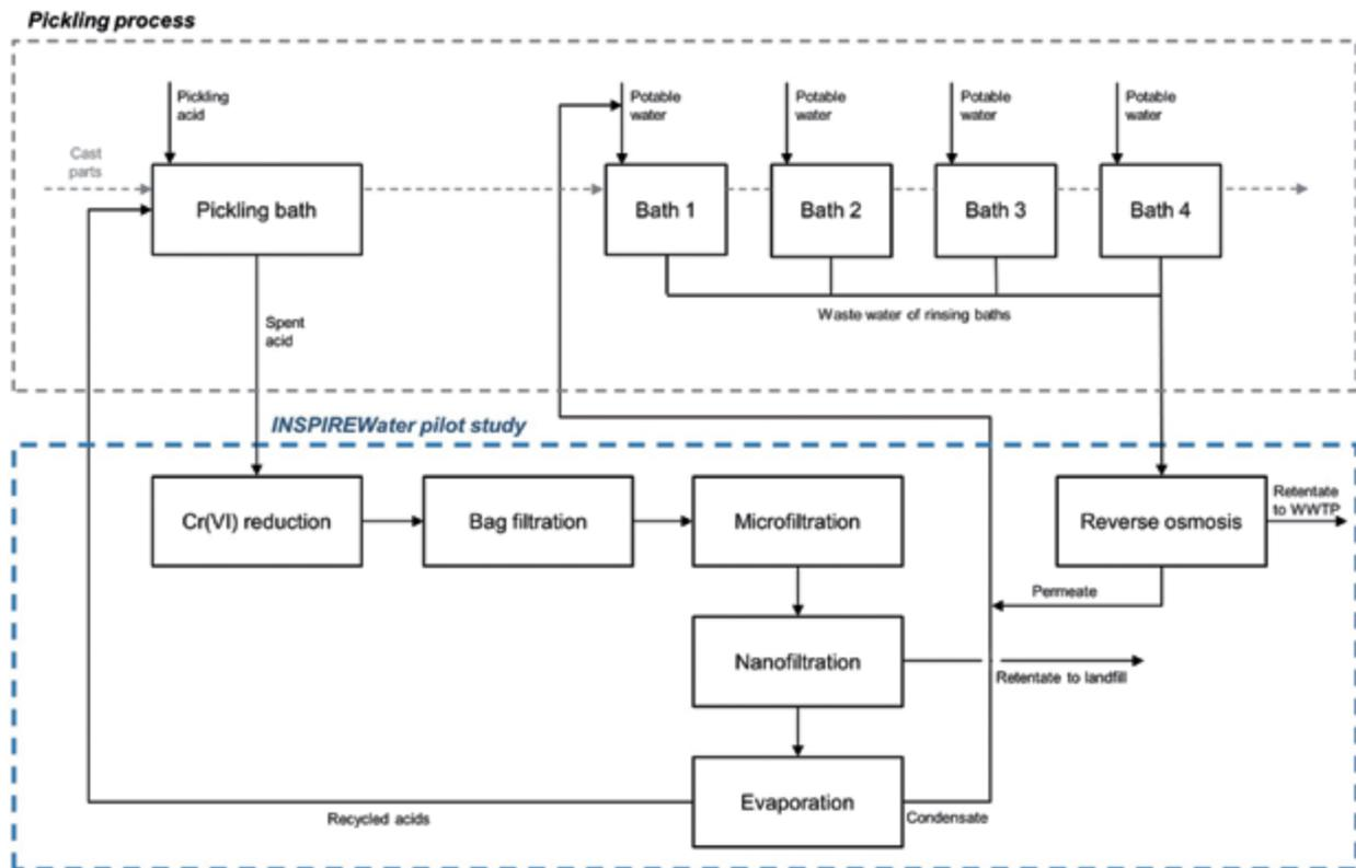
Figure 2: The closed loop recovery system for both pickling acid and rinse water at the SANDVIK demonstration case.
