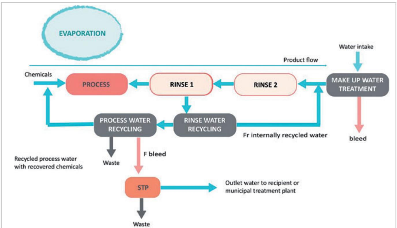
Figure 4: Example of a production process with high water usage. In the figure the light blue arrows are representing water flows with more or less contamination of process fluids, while the dark arrows represent flows with high amount of process chemicals.
